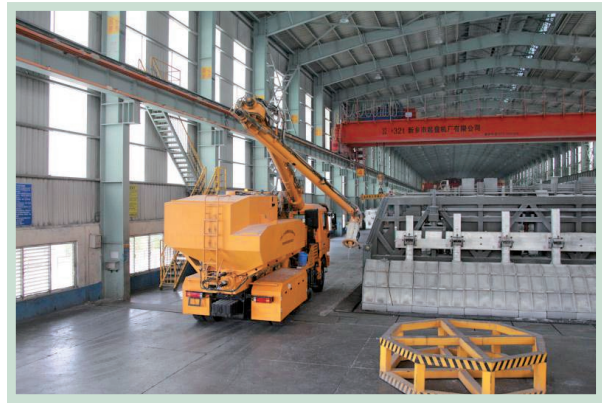
The newly introduced automatic material filling truck
